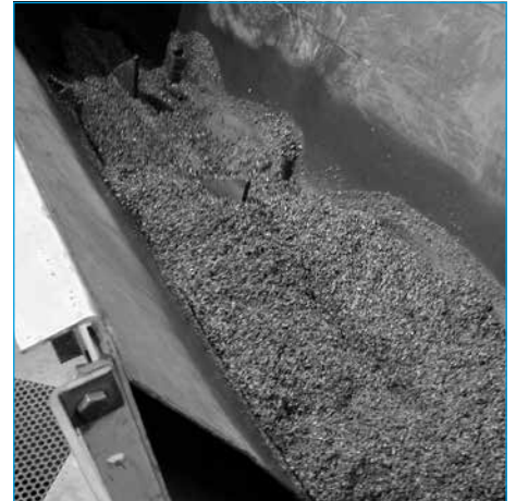
The push-bar centres automatically on the floor of the conveyor trough.
