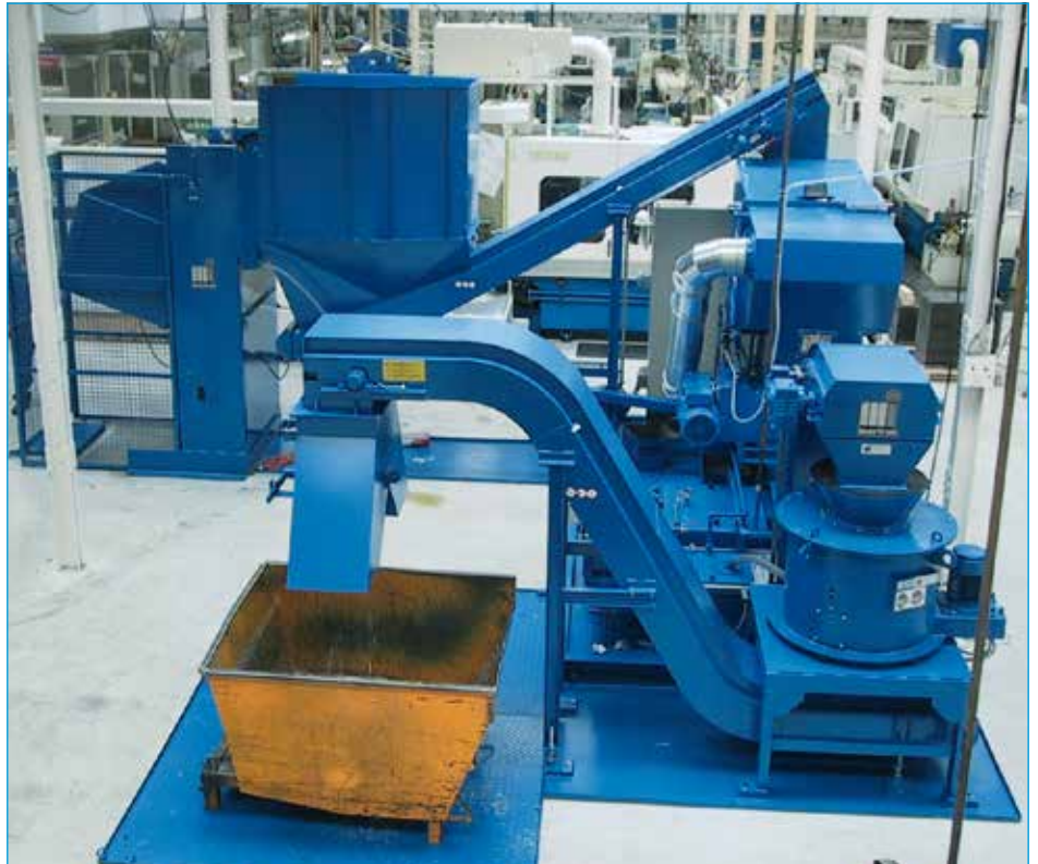
The system consists of the following components: centrifuge, chip crusher, conveyor and container loading.
