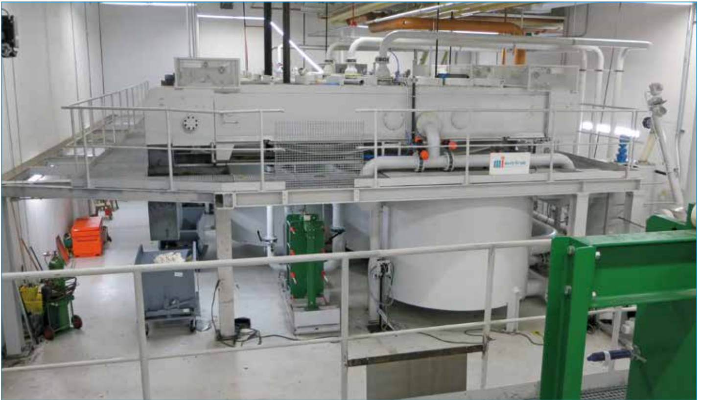
Pressure belt filter system consisting of several filter modules
